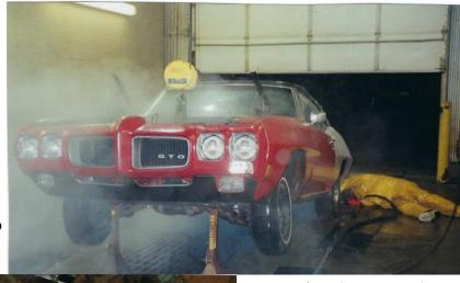
I found some rust by the front body mount at the firewall and determined the only way to fix it properly was to pull the body off the frame. The body mounts looked pretty bad anyway, so I decided to go ahead and replace them all. I started the process of removing fenders, steering column, brake booster and all the wiring and steel lines under the hood. I removed the fuel tank, doors, deck lid and the dash and all
